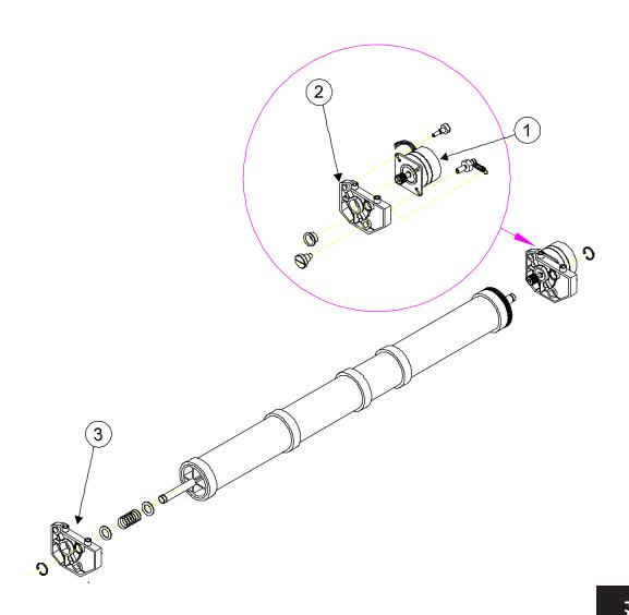
Figure 6-5. Lower Roller Assembly Breakdown.
